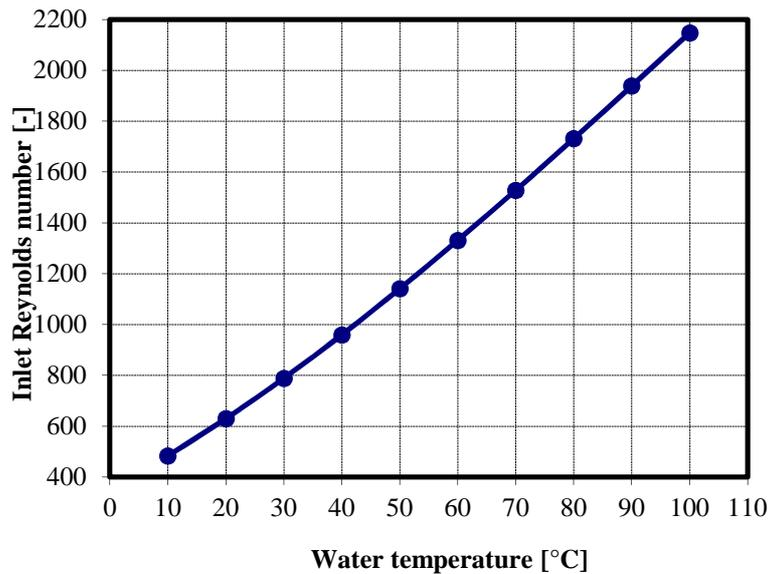
Figure 2: Inlet Reynolds number ( $Re_i$ ) vs. water temperature
